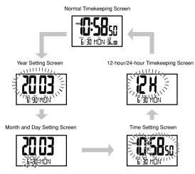
2. While the screen you want is on the display, use the Alarm Time Set buttons (2) to change the digits that are
